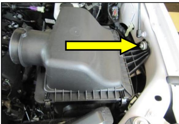
5. Remove the 8mm fender bolt in the air box and remove the entire air box/scoop assembly from the vehicle. **NOTE: On vehicles equipped with a wiring harness attached to the airbox, be sure to unclip the wiring harness from the air box before removal.**
