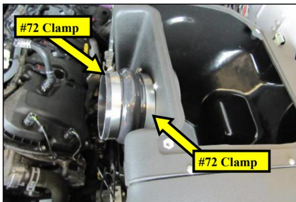
16. Slide the Hump Hose and #72 Clamps onto the Filter adapter, as shown.
